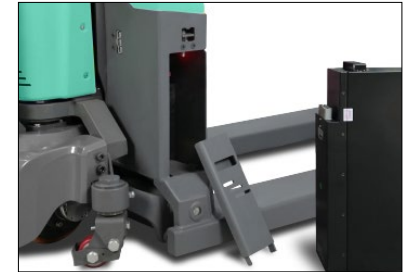
#4 The side-ways battery design allows for the use of various different capacity batteries, ranging from 24V, 25Ah to 24V, 60Ah.
